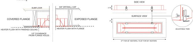
WARNING: Frame and heaters cannot be mounted on a sloped/pitched ceiling. Frame is only to be used on a flat, non-sloped ceiling. Flush mount applications must always be installed with heaters horizontal to the floor
