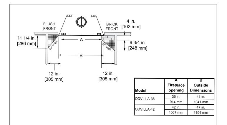
Figure 11.11 Mantel Leg or Wall Projections (acceptable on both sides of opening)
