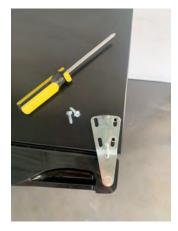
3. Carefully open fridge door and lift fridge door upward off of bottom hinge.
