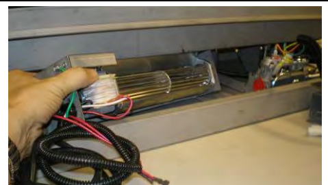
3. Insert fan and place at right rear corner of unit. See Component Locations Section in manual.
