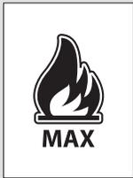
**Flame Height:** Six flame height levels are available. While the flame height icon is displayed, pressing the up or down button once will increase or decrease the flame height by 1 of 6 levels.
