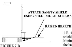
**NOTE:** For raised hearth, safety shield must be under cabinet (See Page 8, Figure 7-A). Also shield must cover any face of combustible material supporting cabinet where hearth connects. (See Figure 7-B)
