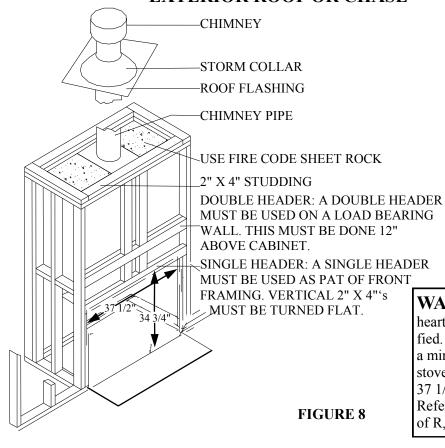
WARNING: Install the hearth protector only as specified. The extension must extend a minimum of 16" in front of the stove door opening and must be 37 1/2" wide minimum.
