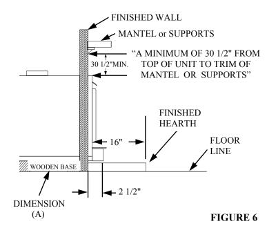
**WARNING:** Install the hearth protector only as specified. The hearth extension must be a minimum of 16" in front of the stove door opening and must be 37 1/2" wide minimum. (See page 6)
