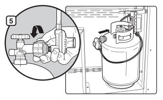
▲ WARNING: Do not use a wrench to loosen the connection. Using a wrench could damage the regulator coupling and could cause a leak. ▲ WARNING: Make sure that all parts are assembled and hardware is fully tightened before operating the grill. Your actions, if you fail to follow this Product Warning, may cause a fire, an explosion, or structural failure resulting in serious personal injury or death as well as damage to property.
