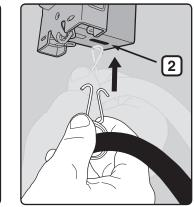
▲ WARNING: The hose must be secured to the tank scale with the Hose Retention Clip. Failure to do so could cause damage to the hose resulting in a fire or explosion which can cause serious bodily injury or death, and damage to property.
