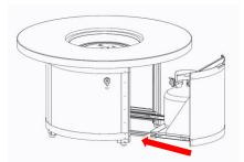
**NOTE:** Over time the bearings in the door glides may require Re-greasing. Perform re-greasing once a year to maintain the smooth operation of the slides. To re-grease the slides, spray any spray lubricant, such as WD-40, into the bearings as you slide the drawer back and forth.
