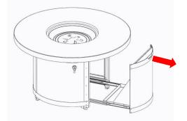
• Tilt propane tank and lower into drawer from the side.
