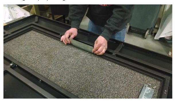
**2.** Using 4 #8-1/2" Phillips head self-tapping screws, secure mounting brackets Part #90293 to Montego top as shown.
