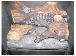
Place the hole in the underside of log #3 onto the locating screw, on the right side of the burner. The bottom branch of log #3 sits in front of, and against, the right end of log #2.
