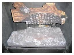
**A.** Place the rear log, as shown, onto the rear log support brackets. Bend the bracket on the right side to help retain the rear log against the back of the firebox.
