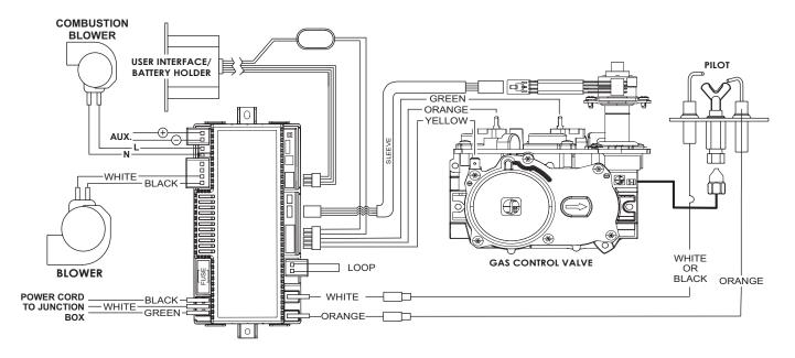
If any of the original wire as supplied with this fireplace must be replaced, it must be replaced with equivalent gauge and temperature rated wire.
