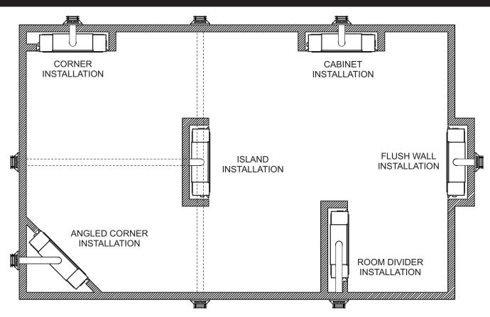
**NOTICE:** Island and Room Divider installation is possible as long as the horizontal portion of the vent system does not exceed 20 feet with a minimum vertical run of 8 feet. See details in Venting Section.
