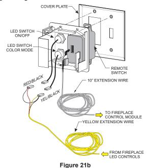
Place batteries in remote receiver and in the remote control using instructions provided. Place the switch slider to the remote switch. Set the remote switch in wall box to remote. (center position) **See Figure 21c.**
