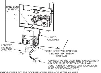
**NOTICE:** OUTER ACCESS DOOR REMOVED. REPLACE AFTER ALL WIRE AND GAS CONNECTIONS HAVE BEEN MADE.
