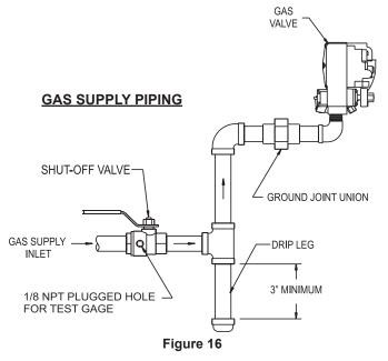
**Installing a New Main Gas Shut-Off Valve (Check Local Code)** Each fireplace should have its own manual gas shut-off valve. A manual main gas shut-off valve should be located in the vicinity of the fireplace. Where none exists, or where its size or location is not adequate, contact your local authorized installer for installation or relocation.
