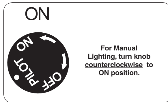
Fig. 11-3 Control knob detail (ON)
